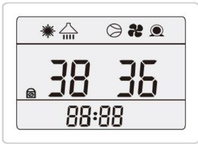
Heating+ DHW status
